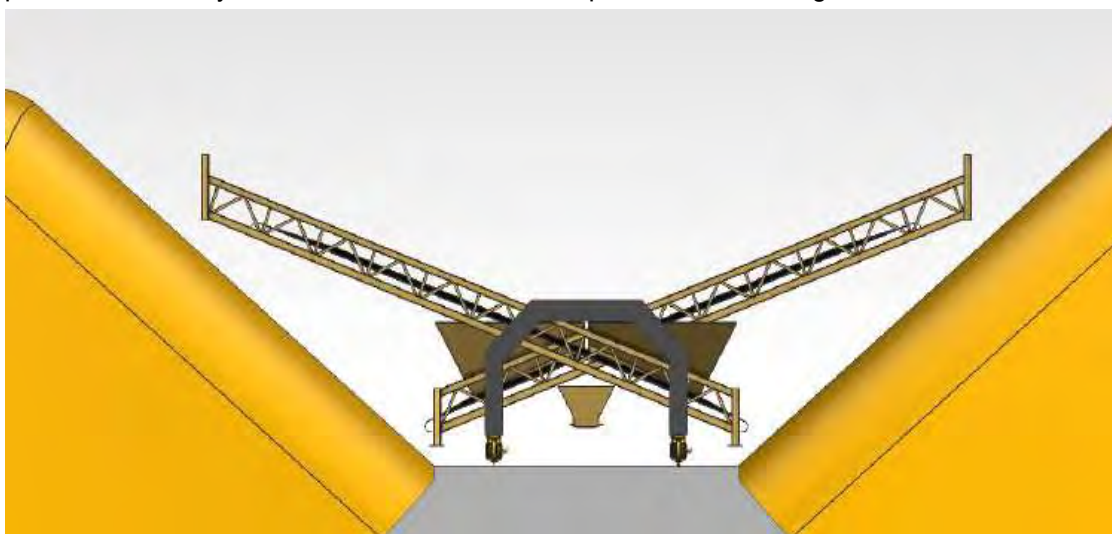
Figure 5 Retracted conveyors clear stockpiles
